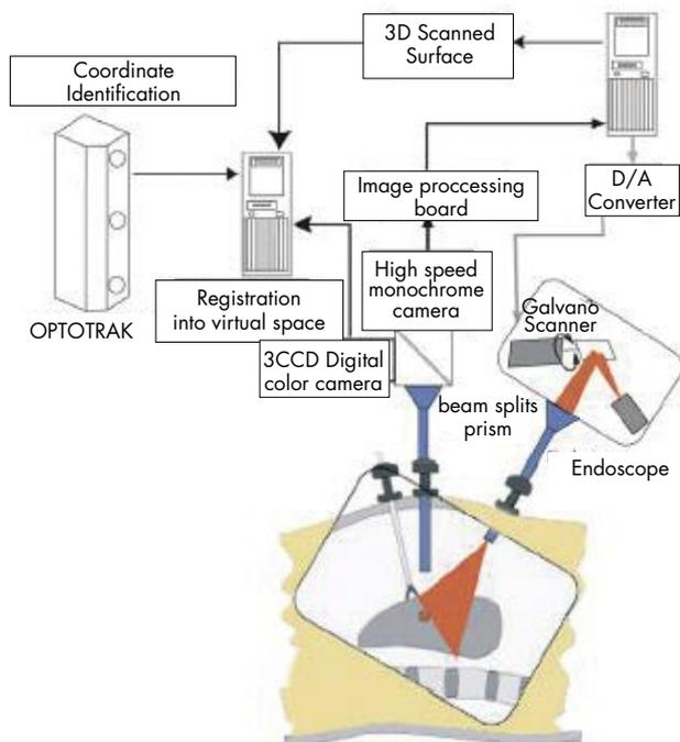
FIGURE 7. Scan Laser endoscope: System configuration (By courtesy of Prof. Hayashibe. Tokyo University, Japan).
