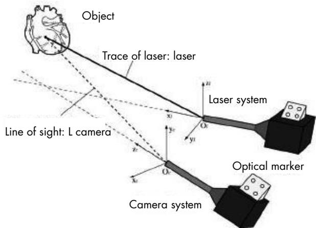
FIGURE 6. Laser-camera coordinated system scheme (By courtesy of Prof. Hayashibe. Tokyo University, Japan).
